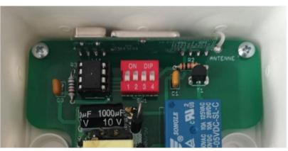
Since it is possible to install multiple control devices in a single house which should switch independently from one another, each system must transmit on its own channel (similar to WiFi networks). In apartment buildings too, it can be the case that each apartment has their own system. You can now select from among 4 channels which are set using the switches shown above so that the control device now only switches the radio receivers which are also part of the system, and not all of them.
