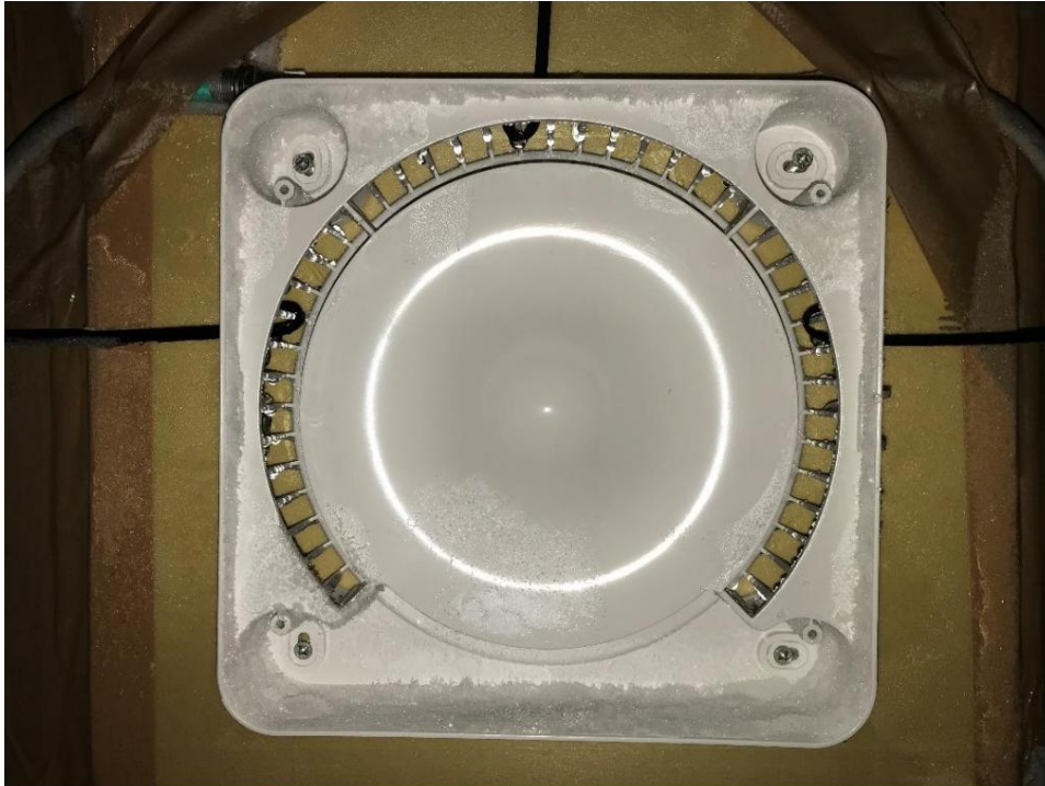
Figure H-1: Device without external cover after the end of the test
